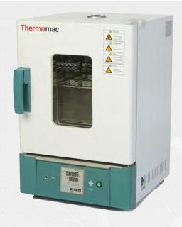
The device uses physical method to achieve disinfection and sterilizing. It takes advantage of high-temperature and hot air to cause intoxication on microbial oxidation, protein denaturation, and electrolyte concentration. By disinfection principle, it destroys protoplasmic cell to kill all the microorganisms in a certain period of heating time.
