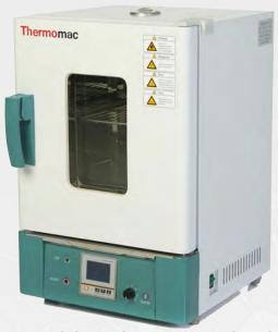
This new device is widely used for drying, baking, soluble wax, solidification and thermal treatment in the school laboratory, industrial and mining, food processing, biochemistry, agriculture, and pharmaceuticals industry for the samples.
