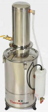
This series of apparatus have tap water as source to produce pure water by electrical heating distilling. It is applied in health and medicine units, chemical industries, scientific research institutions and labs etc.
